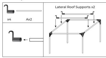
8. Create the Lateral Roof Supports by sliding the Lateral Roof Support Clamps x4 onto the ends of A Poles x2. Attach them to the top of the tent frame below the Medial Roof Support. Make sure the open part of the clamps face the floor when attaching the supports.
