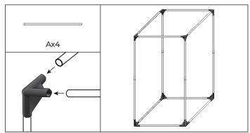
6. Start building the top of the tent using A Poles x4. Make sure the tent poles are seated firmly in Corner Connectors after inserting.
