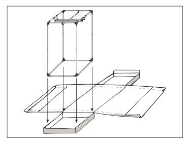
9. Unzip all zippers before covering the framing with the tent. Spread the tent on the ground and put the tent frame into the bottom of the tent covering.
