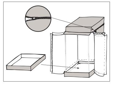
11. Zip all tent seams together and insert the spill tray into the bottom of the tent. Use the velcro straps on each corner of the spill tray to attach it to the tent's corner poles.
