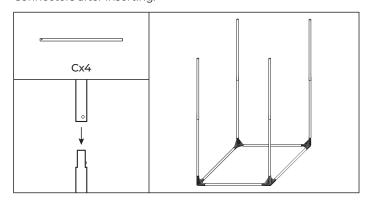
4. Add another section of vertical poles using C Poles x4. Make sure the bearings on B Poles align correctly with the holes on C Poles and snap into place.
