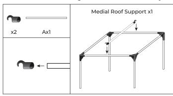
7. Create the Medial Roof Support by sliding the Medial Roof Support Clamps x2 onto the ends of A Pole x1. Attach it to the top of the tent frame in the center. Make sure the open part of the clamps face the floor when attaching the support.
