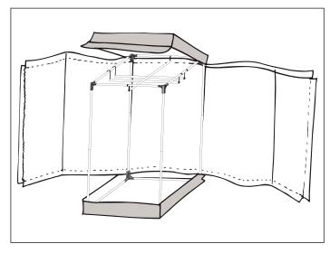
10. Place the tent covering over the top of the tent frame and continue to wrap the sides and front of the frame. Note do not use excessive force when stretching the tent covering over the frame.
