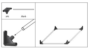
2. Build the bottom of the tent using Corner Connectors x4 and A Poles x4. Make sure tent poles are seated firmly in Corner Connectors after inserting.
