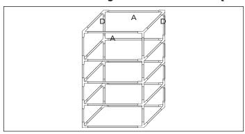
6. Build the top of the tent using 3-Way Corner Connectors x4, A Poles x2 and D Poles x2. Make sure tent poles are locked firmly in Corner Connectors after inserting.
