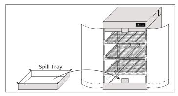
11. Insert the spill tray into the bottom of the tent. Use the velcro straps on each corner of the spill tray to attach it to the tent's corner poles.
