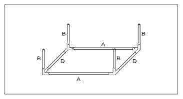
2. Build the bottom of the tent using 3-Way Corner Connectors x4, A Poles x2, D Poles x2 and B Poles x4. Make sure tent poles are locked firmly in Corner Connectors after inserting.
