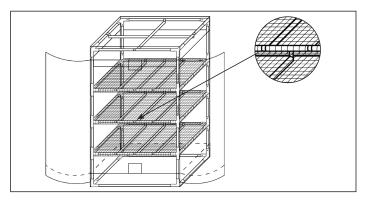
10. Build the tent shelving using Shelving Sections x6 (2 per shelf). Place each shelf section over the shelf frame poles. Make sure to adjust the medial shelf supports if needed to line up with the openings on each shelf.
