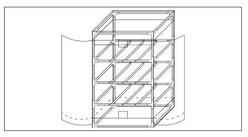
8. Add the medial shelf supports to each shelf using E Poles x9 (3 per shelf). Note: Supports must be spaced to fit the openings on each shelf.
