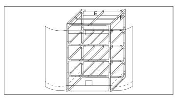
9. Add the medial and lateral roof supports using E Pole x1 and F Pole x1.
