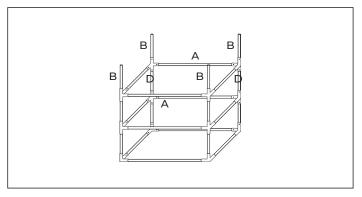
4. Build the middle shelf frame using 4-Way Corner Connectors x4, A Poles x2, D Poles x2 and B Poles x4. Make sure tent poles are locked firmly in Corner Connectors after inserting.
