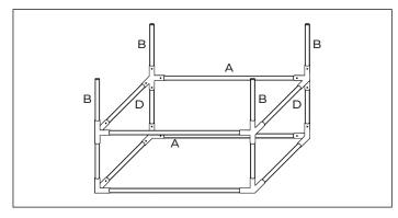
3. Build the bottom shelf frame using 4-Way Corner Connectors x4, A Poles x2, D Poles x2 and B Poles x4. Make sure tent poles are locked firmly in Corner Connectors after inserting.
