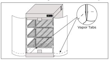
12. While zipping the tent seams together, make sure all Vapor Tabs are tucked inside the tent doors and hanging over each side of the spill tray. This will ensure excess water buildup on the tent walls drains into the spill tray instead of the tent floor. Note: If the Vapor Tabs are not tucked inside the tent, the doors will not close.
