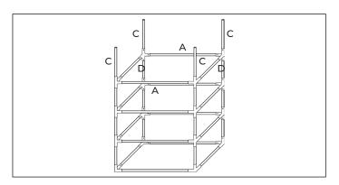
5. Build the top shelf frame using 4-Way Corner Connectors x4, A Poles x2, D Poles x2 and C Poles x4. Make sure tent poles are locked firmly in Corner Connectors after inserting.
