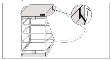
7. Unzip the tent canvas completely. Pull the canvas over the top of the tent frame first. Next, pull the canvas over the bottom of the tent frame. Tip: Lay the tent frame on the ground horizontally while adding the canvas to make installation easier. Doors may also be secured using the velcro straps on the top of the tent. Do not use excessive force when stretching the canvas over the frame.
