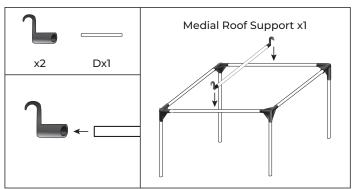
8. Create the Medial Roof Support by sliding the Medial Roof Support Clamps x2 onto the ends of D Pole x1. Attach it to the top of the tent frame below the Lateral Roof Support. Make sure the open part of the clamps face the floor when attaching the support.
