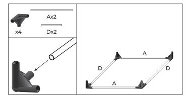
2. Build the bottom of the tent using Corner Connectors x4, A Poles x2 and D Poles x2. Make sure tent poles are seated firmly in Corner Connectors after inserting.
