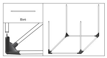
3. Slide B Poles x4 into existing Corner Connectors. Make sure tent poles are seated firmly in Corner Connectors after inserting.
