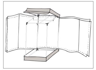
10. Place the tent covering over the top of the tent frame and continue to wrap the sides and front of the frame. Note do not use excessive force when stretching the tent covering over the frame.
