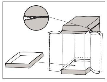
11. Zip all tent seams together and insert the spill tray into the bottom of the tent. Use the velcro straps on each corner of the spill tray to attach it to the tent's corner poles.
