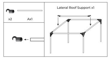
7. Create the Lateral Roof Support by sliding the Lateral Roof Support Clamps x2 onto the ends of A Pole x1. Attach it to the top of the tent frame in the center. Make sure the open part of the clamps face the floor when attaching the support.
