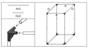
6. Start building the top of the tent using A Poles x2 and D Poles x2. Make sure the tent poles are seated firmly in Corner Connectors after inserting.
