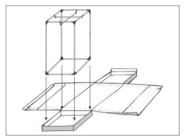
9. Unzip all zippers before covering the framing with the tent. Spread the tent on the ground and put the tent frame into the bottom of the tent covering.
