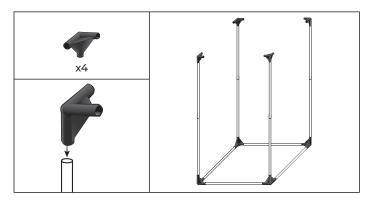
5. Slide Corner Connectors x4 on top of C Poles. Make sure tent poles are seated firmly in Corner Connectors after inserting.
