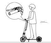
Hold the brake handle and lightly step on the rear fender to assist braking.
