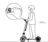
Press the accelerator to speed up and turn the grip to adjust the direction.
