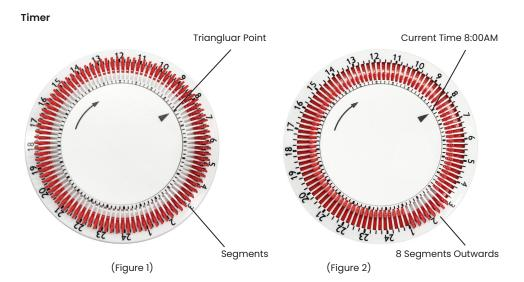
The heater can be set to turn ON and OFF at specific times of the day. There are 96 segments around the dial. Each of these segments represent a 15-minute time period.
