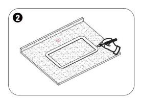
Place the cardboard mold on the counter, and determine the installation positions for the faucet and basin according to the installation requirements for the supporting faucet. Use a pencil to draw the auxiliary line.
