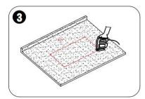
Use the cutting machine or electric drill to make holes along the auxiliary line, and sand the edge of the holes.
