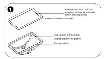
Make the cardboard mold according to the pasting surface of the basin.
