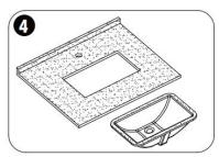
Use the cutting machine or electric drill to make holes along the auxiliary line, and sand the edge of holes. Place the cardboard mold to the bottom of the counter, use a pencil to draw the auxiliary line. Apply special glue water on the contact area of the basin and counter, and then paste the basin along the auxiliary line with tighgtness (let it dry for 24 hours).
