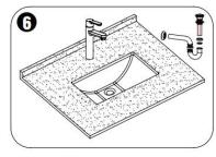
Install a lever faucet on the basin. Install the faucet and its components.
