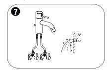
Connect the water supply pipe to the faucet, and carefully bend the pipe to make it match the water supply shut-off valve. Ensure the pipe is sealed. (Always wash the sediments in the water supply pipe away before connecting the angle stops
