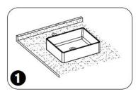
Place the basin on the counter, and determine the installation positions for the faucet and basin according to the installation requirements for the supporting faucet.
