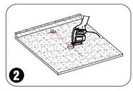
Mark the faucet and basin at the determined installation positions with a pencil, use the cutting machine or electric drill to make holes, and then sand the edge of the holes.
