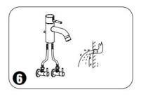
Connect the water supply pipe to the faucet, and carefully bend the pipe to make it match the water supply shut-off valve. Ensure the pipe is sealed. (Always wash the sediments in the water supply pipe away before connecting the shut-off valve.)
