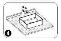
Apply mildew-proof neutral glass cement on the contact area of the basin bottom part and counter, place the basin properly on the surface, and then firmly press it (let it dry for 24 hours).
