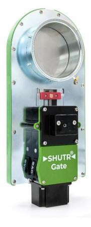
The Gate complies with CE/ATEX 114, internally for zone 21, externally zone 22, meaning that it can be used for certain explosion hazardous applications such as dust collection systems. The electronics housing is made of strong, UV-proof polycarbonate and fully sealed to level IP54, dustproof. The antenna for wireless operation is located inside the electronics housing. A brushless, maintenance free motor drives the slide.
