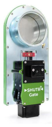
The Gate complies with CE/ATEX\*\*, internally for zone 21, externally zone 22, meaning that it can be used for certain explosion hazardous applications such as dust collection systems. The electronics housing is made of strong, UV-proof polycarbonate and fully sealed to level IP54, dustproof. The antenna for wireless operation is located inside the electronics housing. A brushless, maintenance free motor drives the slide.
