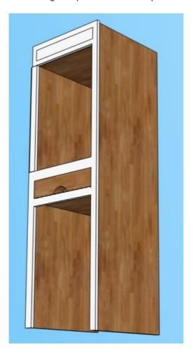
Slide the pull out shelf in and adjust with the adjustment below the shelf on the runners.
