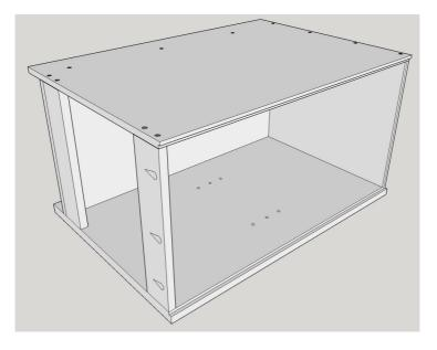
Once in go around and screw the side to the base, back and top bars in all the pre marked places.
