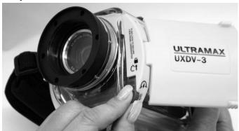
Push the RED Locking Knob upwards to secure the Mirror View Panel in place and prevent it from flipping back underwater due to the resistance of the water current (Slightly flip the view panel backwards during push-to-lock process if you found it difficult to lock the Locking Knob)
