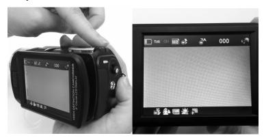
KEEP ON pressing the "Playback" button and then press the "Shutter" button for approx. 3 seconds until the image & all icons are displayed in "mirrored" images
