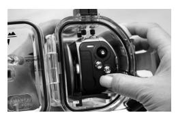
MAKE SURE to TURN ON the DV Camera, slide the DV Camera into the underwater housing thru the "Guiding Slot" of the housing until it was fully inserted and securely seated
