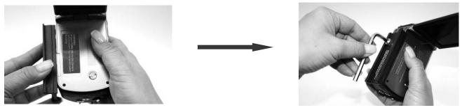
Position the "Support Tray" to the mounting hole of the DV Camera, tighten the screw using the hexagon key provided. Make sure the "Support Tray" is straightly aligned with the DV Camera
