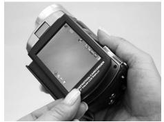
Flip the LCD Panel back to the original position with the display facing outward
