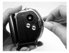
Tie in the "Pulling Strap" to the strap hole for pull out convenience of the DV Camera
