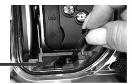
Place the "Pulling Strap" buckle underneath the support tray
