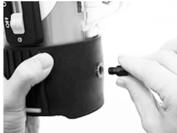
Step 4 Connect the other end of the Optic Cable Jacks to your external flash
