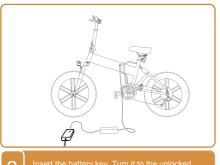
2 Insert the battery key, Turn it to the unlocked position.
