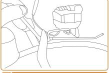
Re-install the light facing forward: Keep the washer between the bolt head and light holder and then tighten the bolt with a hex key and a wrench.
