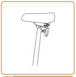
Close the seatpost clamp and make sure the seatpost is held in place. Don't adjust he seat too high (keep the safety line mark lower than the top of the seat tube).
