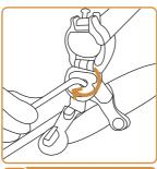
Tighten the bolt into the head tube.
