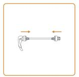
3 Loosen the adjusting bolt of the QR skewer, Make sure the smaller end of the 2 cone springs facing inwards
