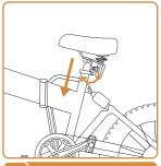
Loosen the seat clamp and adjust the seat to an appropriate angle.
