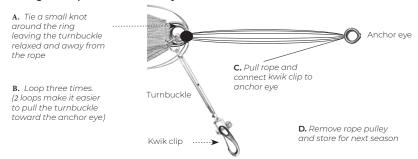
**NOTE:** The location of nuts are away from the body on the turnbuckle. This will enable you to spin the turnbuckle body to tension the turnbuckle once your sail is attached. Be sure to orient yourself with the tightening of the turnbuckle by spinning the body. **Be sure not to spin the turnbuckle the wrong way as it will come apart.**
