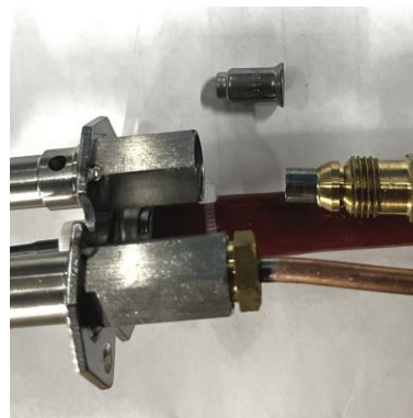
Figure 9.3 – Cleaning pilot orifice
