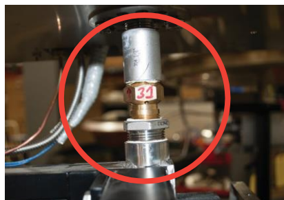
Figure 9.1 – Locating orifice for cleaning.
