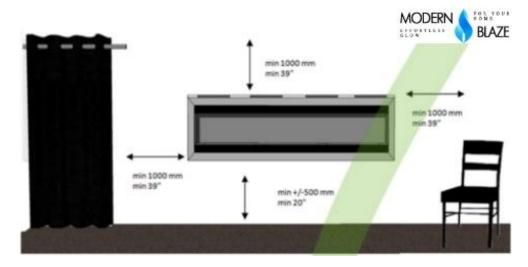
The above diagram shows the most common clearance requirements for recessed ethanol fireplaces.
