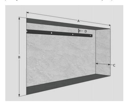
Generally, your finished opening should be 4" wider and 2-1/2" higher than the back of the fireplace (including burners hanging from the bottom of the fireplace). This extra space allows for faster installation, air circulation and provides an escape for the hot air.
