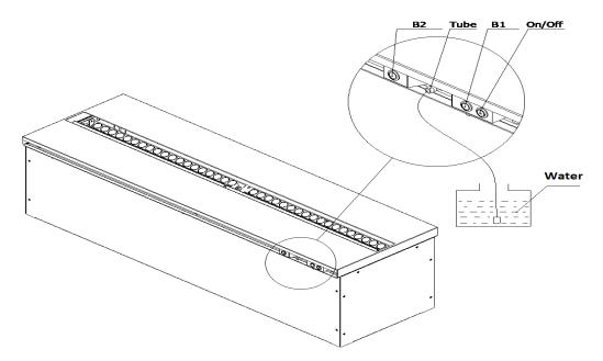
**The ON/OFF button** turns the device on and off. **Button B1** is used to fill the reservoir with water. **Button B2** is used to empty the device. **Hold the button for 5 seconds to start the pumps**. Press once to stop the pumps. The stainless-steel "Tube" connection connects to the plastic hose provided to fill and empty the device.
