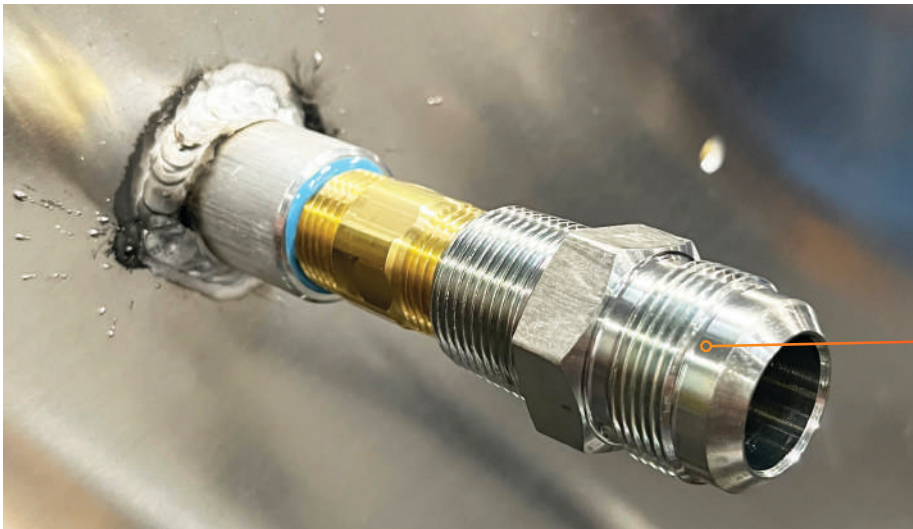
Photo 17: Attaching the Male Flare Hose Adapter
