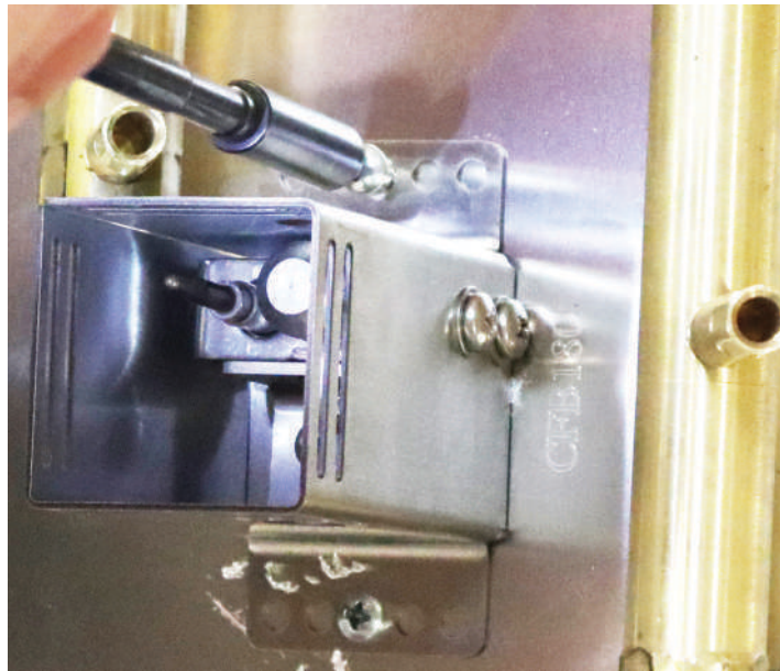
Photo 5: Securing the Pilot to the Plate/Pan
