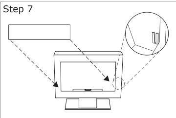
Insert glass panel into the slots located on the inner sides of the fireplace.
