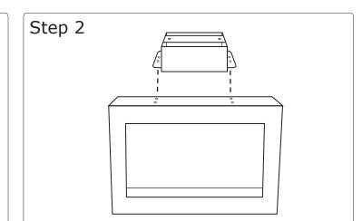
Turn your fireplace upside-down onto its top and place the stand (Part H) onto the fireplace. Make sure the flanges that stick out line up with the 4 holes pre-drilled in the fireplace.
