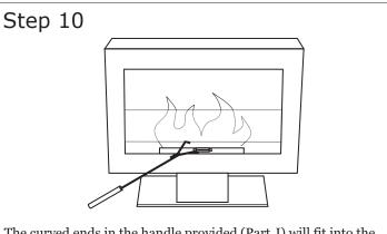
The curved ends in the handle provided (Part J) will fit into the holes in the lid of the burner. You can adjust the flame height to get the desired flame height and heat output. When you are ready to extinguish the fireplace, use the handle to slide the lid of the burner completely closed over the opening to cut off the oxygen supply to the fuel. This will snuff out the flame.
