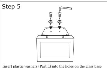
Insert plastic washers (Part L) into the holes on the glass base (Part I) and secure the glass base onto the stand using the thick .75" screws (Part M) using the hex tool provided. Be sure not to over tighten. Until screws are secured, glass may not be stable. Be careful and insure that glass base does not fall before securing.
