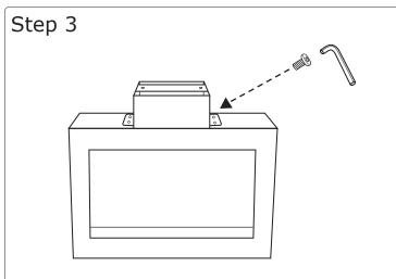
Attach the stand to the fireplace frame using the 4 .5" screws (Part K) using the provided hex tool.
