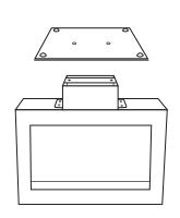
Now place the black glass base (Part I) over the stand so that the holes in the glass line up with the holes on the bottom of the stand. Make sure the rubber feet on the glass base are facing you. This will become the bottom of the fireplace.
