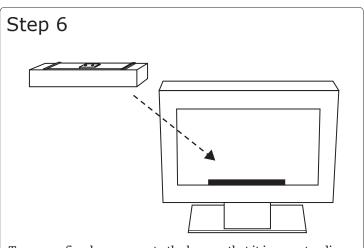
Turn your fireplace over onto the base so that it is now standing right side up and place the burner (Part B) into the recessed hole in your fireplace frame.
