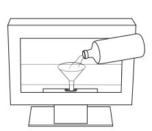
Using the funnel provided, (Part N), carefully pour in the liquid ethanol fuel for fireplaces into the burner about <sup>3</sup>/<sub>4</sub> full. Make sure you do not over fill the burner. If any fuel does spill, you should always wipe it up prior to lighting your fireplace.
