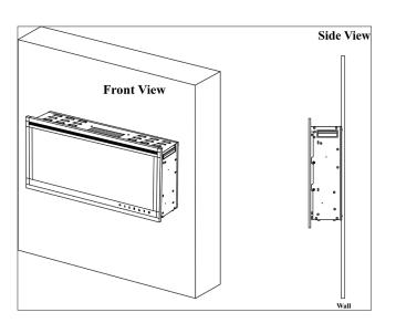
2. **Built in Installation.** Appliance is built inside the wall or cabinet. It is great for remodeling project and new construction site as it requires certain amount of wall modification, framing and reframing work such as cutting an opening in a wall, building and framing a stud wall out, and electrical wiring.
