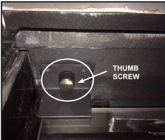
Figure 4.12 Glass Removal and Installation
