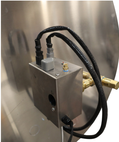
Photo 11: Electronic Connections from the Pilot to Valve
