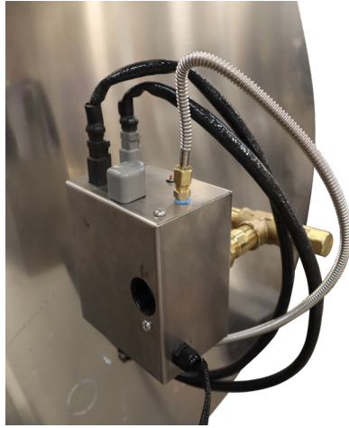
Photo 12: Connecting the Gas Line From the Pilot to the Valve
