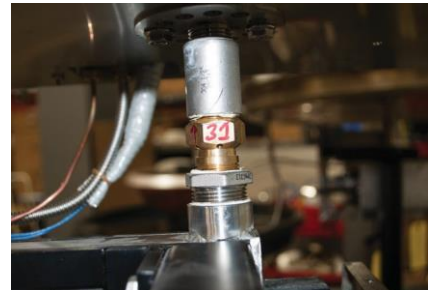
Figure 10.1 – Locating orifice for cleaning
