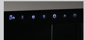
TOUCH SCREEN CONTROL PANEL WITH MOTION PROXIMITY SENSOR
