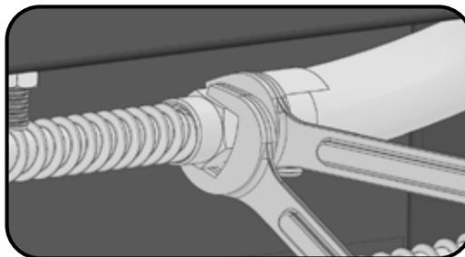
**Reinstallation:** Reverse the procedure to reinstall the burner tray. Check that the orifice enters the burner when installing. Replace the glass embers and the front glass shield. When the appliance is put back in service, compare the burner flame pattern to the images in the “Operation” section to verify that the appliance is operating correctly.
