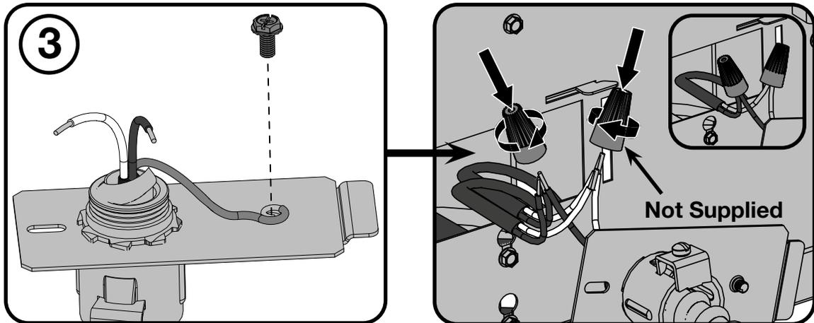
4. Re-install the cover plate using the screw (N570-0008), as shown.
