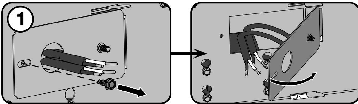
2. Install the box connector through the 7/8" (22.2mm) hole and into the junction plate.
