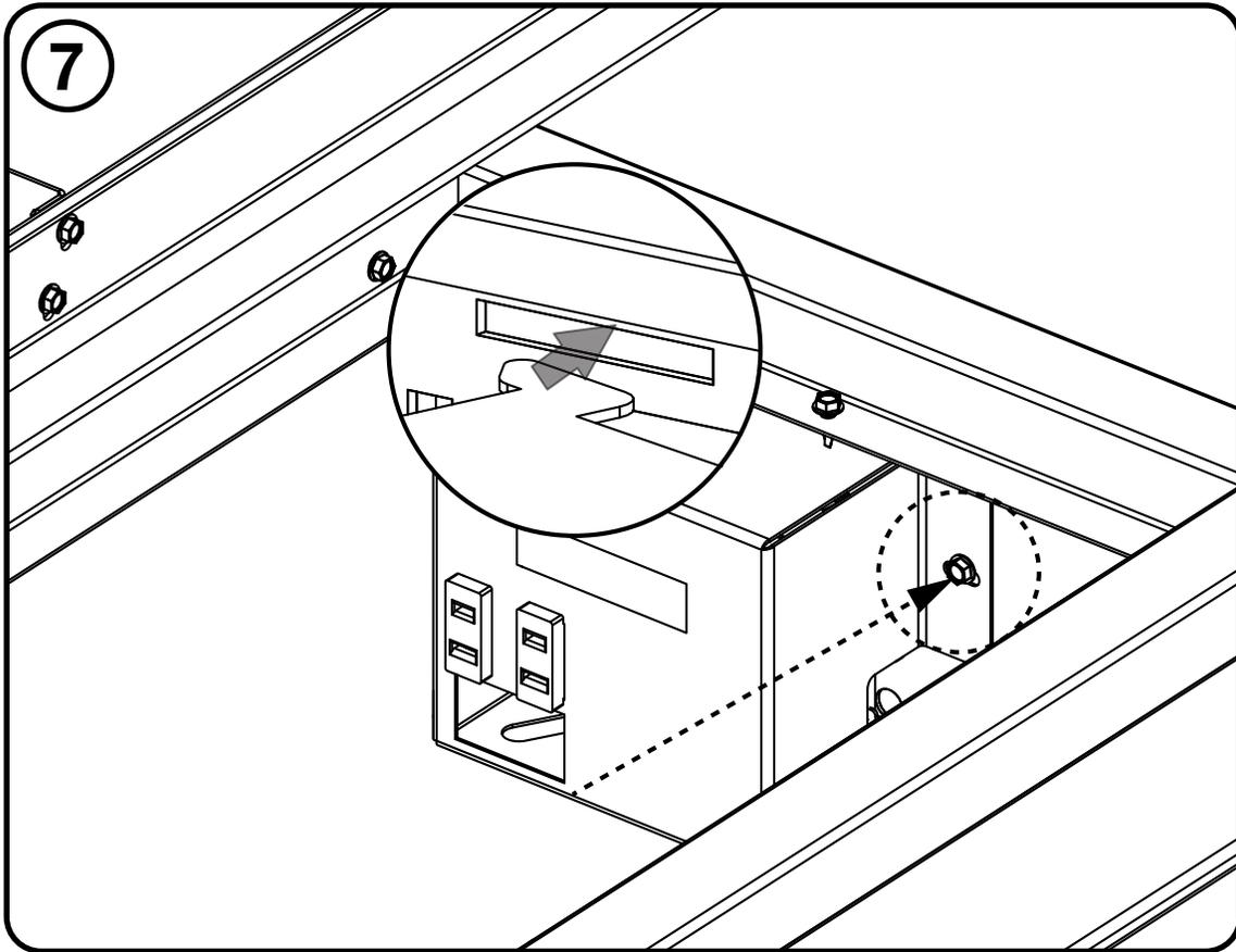
8. Re-install the burner tray with the handles as illustrated. Take care not to damage pilot tube and wires.
