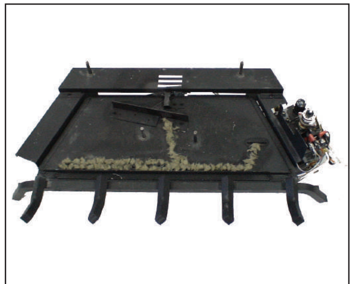
Figure 6.2 - Correct Rock Wool Placement
