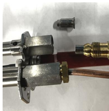
Figure 9.3 – Cleaning pilot orifice
