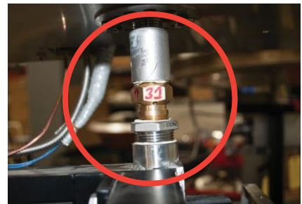
Figure 9.1 – Locating orifice for cleaning
