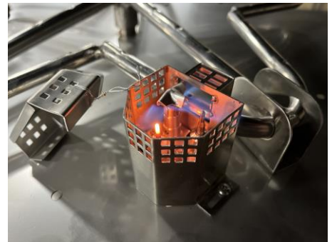
Figure 9.2 – Pilot flame coverage of thermocouple.
