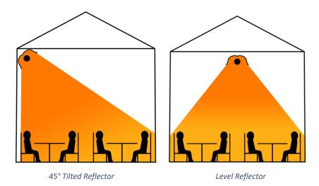
**Image 3.** Our heaters are shipped with hardware that allows for level or tilted installation. When mounted on a wall, installing at an angle directs the heat more efficiently for diners.
