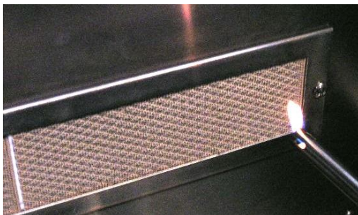
Manual Lighting of Infra-Broil Rear Burner
