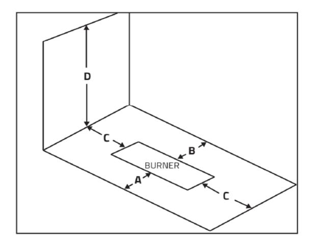
IMPORTANT: If the burner install in a single side openning fireplace surrounding, please make the MAX DEPTH of the fireplace 20 inches, if too deep the fireplace is, it's not good for heat/air circulation. If it's install in a double side openning or all open fireplace surrounding, then free to the depth size.
