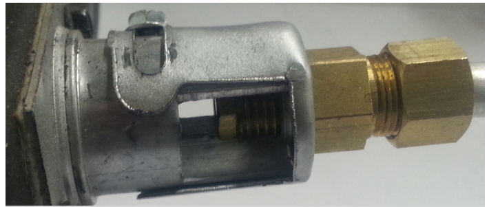
NOTICE: Orifice shield removed for photo quality. Figure 3 - Air Shutter Fully Open
