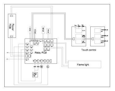
The unit is hardwired and has no main switch. (Caution: If servicing this unit, turn off power at the main circuit breaker.) An optional tethered wall control switch is included, refer to installation instructions to relocate the tethered wall control switch to a wall location.
