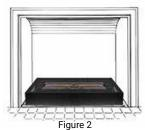
Place Bedrock burner in your fireplace centering the base front to back and side to side. Centering the base allows the case to easily slide over the top of the base. (Figure 1)
