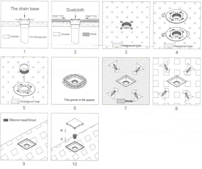
STEP1. Coupling the drain base outlet to 2" schedule 40 DWV pipe using correct solvent cement. STEP2. Blocking the drain opening with a rag, trowel mortar to build shower pan, reinforce around drain base to be flush with the floor, grade to create MIN 1% slope towards the drain.
