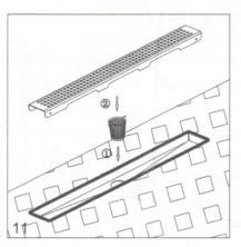
STEP 1. Coupling the drain base outlet to 2" schedule 40 DWV pipe using correct solvent cement.
