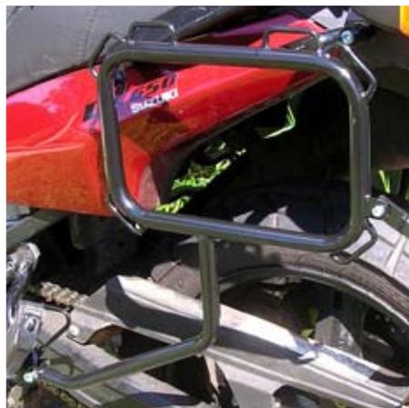
containers. They are made of welded chrome-moly steel with slotted bolt holes for simple, painless installation. High-grade nuts and bolts for mounting are supplied with the complete kit and it's all available online via the AdventureMoto.com.au online store.
