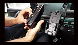
5. Use the provided prongs on the adaptor to tidy up excess cables.
