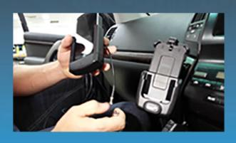
4. Plug the USB cable from the Alpha Cradle into the USB port of the adaptor.
