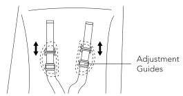
2. To adjust the shoulder belt length, move the adjustment guides up to shorten or down to lengthen.
