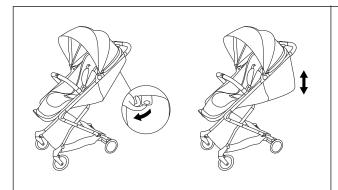
Lift the backrest adjustment lever and adjust the backrest to the most suitable recline position.
