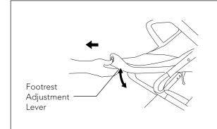
Pull the footrest adjustment lever and adjust the footrest to the most suitable position.
