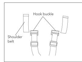
3. To remove the shoulder belt, remove the hook buckle from the shoulder belt.
