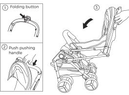
2. Press the folding button ① and push the handle bar ② downwards to fold the stroller according to the direction of the arrow as shown in ③.
