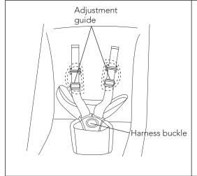
2. To adjust the shoulder and crotch strap length, move the adjustment guides up or down to shorten or lengthen.
