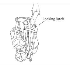
3. Secure the stroller with the locking latch.
