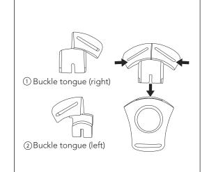
1. Put the left ②and right ①tongues of the buckle together. Ensure the buckle tongues are firmly together. Insert the joined tongues into the harness buckle until you hear a "click" sound. Make sure the harness buckle is secure by pulling the shoulder belt upwards.
