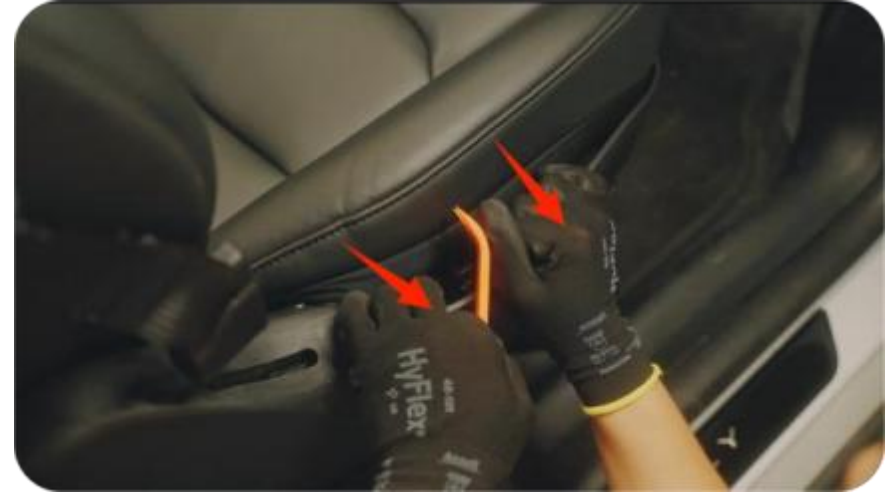
10. Use tools to remove the seat trim panel
