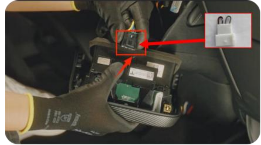
2. Pull out the plug of the charging module, and connect the emergency plug to the charging module. Electrical module plug mating
