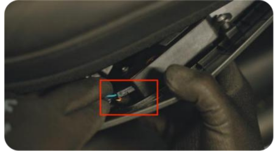
14. Another adapter plug is plugged into the original seat adjustment socket (The same applies to the main driver's seat adjustment adapter cable )
