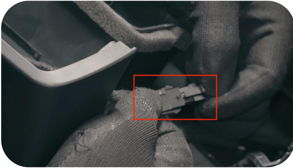
17. Plug in the power harness plug
