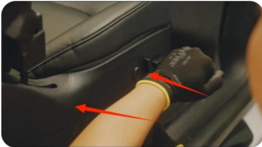
15. Align the correct position and press back
