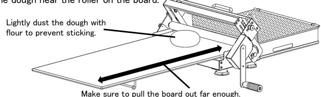
3 While turning the handle, push the sheeter board toward the Curling Chain. (The dough will roll into a cylindrical shape as it passes under the Curling Chain.)
