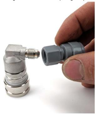
Step 2: Use a marker and mark both the FFL and MFL sides of the fitting.
