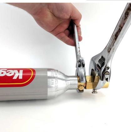
Always use two spanners when tightening or loosening any attachments onto the Sodastream cylinders.
