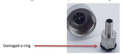
If you are still experiencing issues with the carbonation caps then please send through a video to the email <a href="mailto:beer@kegland.com.au">beer@kegland.com.au</a> showing where the leak is occurring (leak test) and photos of the condition of the carbonation cap and the o-rings.
