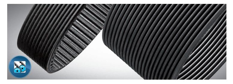
The **optibelt OMEGA RB** differential timing belt features a RB belt ground into the back-side. This creates a unified belt that will not separate. The belts are used primarily in mills where the back pulley has a reversible direction. The RB backside will allow for slippage if the machine becomes blocked or locks-up.
