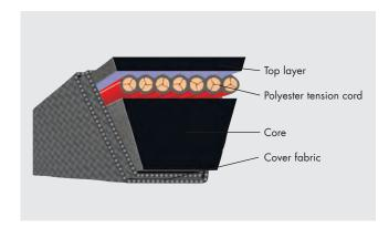
The components used are perfectly suited to the power ratings P<sub>N</sub>. These values are far above those given by DIN 2218. Thus the operational safety in existing drives is increased and overloading is avoided.
