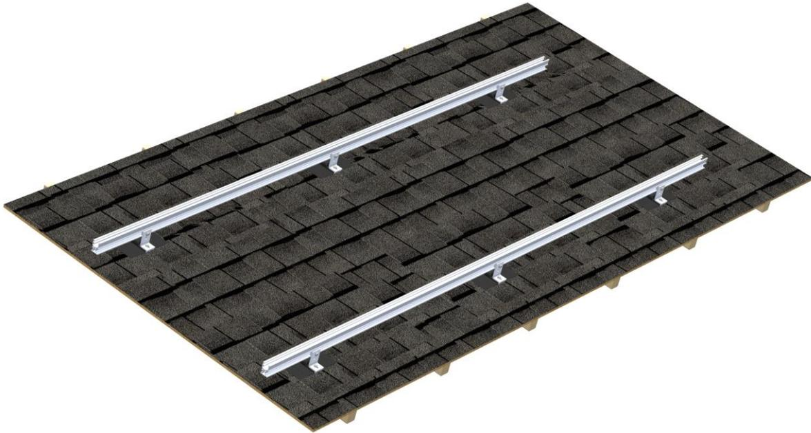
a) Insert the K-Nut of the L-Bracket assembly into the side channel of the rail.
