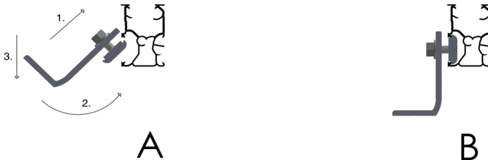
Figure 2: Inserting K-Nut into Side Channel
