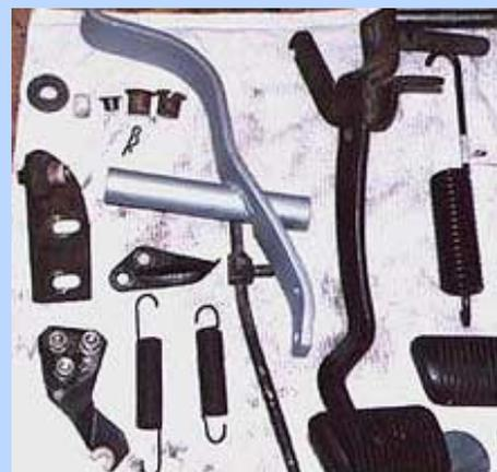
Converting an early Ford from automatic to manual requires rounding up the original clutch activation parts. This can be tough, the best bet is to find a wrecked four-speed car and take everything. Shown here are parts from an early Mustang, including the z-bar
