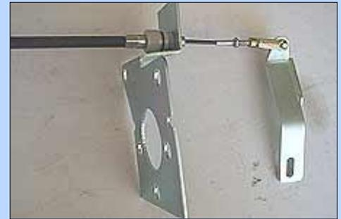
The kit is designed for strength as well as ease of installation. The 1/8" thick steel support plate mounts between the firewall and master cylinder. It not only locates the cable but strengthens the firewall by distributing the brake and clutch pedal loads.
