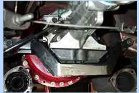
The [Modern Driveline](#) crossmember is a strong piece which follows the stock shape, making for better header and exhaust clearance.
