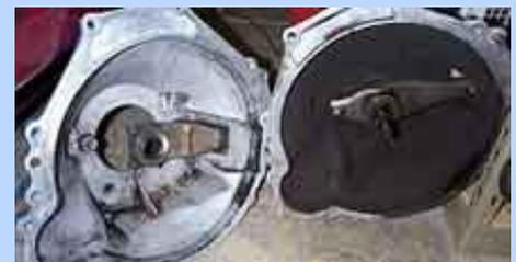
Cable operated clutch fork (right) and converted fulcrum style clutch fork (left.)
