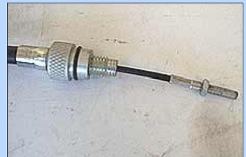
The cable is not an off-the-shelf stock piece as found in some conversion kits, it is a custom spec'd piece with a duel-lined inner cable and an integrated firewall tension adjuster.
