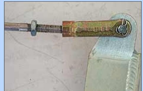
The cable attaches to the clutch pedal using a clevis/pedal bracket. The bracket mounts to the pedal with no modifications, and positions the cable at the highest point above the pedal pivot in order to maximize leverage and minimize pedal effort.
