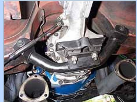
The California Pony Cars T5 crossmember serves its purpose, however the mount bracket welded to the main tube is a weakness. The member also offers less exhaust clearance.
