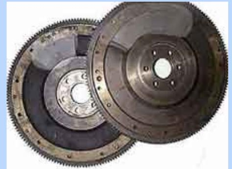
Be sure to use the flywheel which matches your engine balance factor. 289's and early 302's used the 28oz. balance factor, as seen by the smaller counter weight (left.) Late model flywheels used a 50oz. factor (right.)
