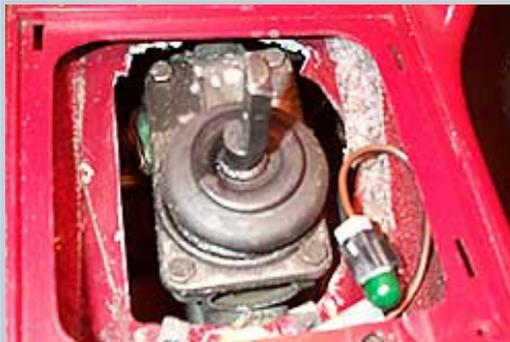
**4** Note that our '88 was originally an AOD car which we [converted to T5](#)(hence the green shifter light and carved up transmission tunnel.)
