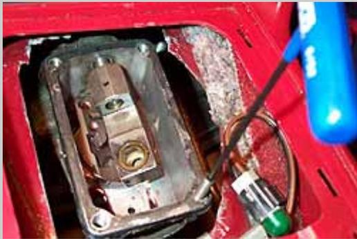
**7** One of the upgraded features of the Pro Ripper is that it mounts using these studs, rather than the stock bolts. Studs are a little stronger than bolts, and it makes for easier installation of the new shifter.
