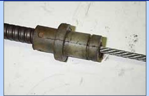
Stock cables, such as this 5.0L unit, use inferior nylon ends and a bare cable which eventually binds and corrodes. The lined cable included in the Modern Driveline kit offers a smooth and virtually frictionless pedal effort.
