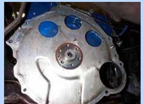
Use the T5 block plate and the late-model 302 pilot bearing.
