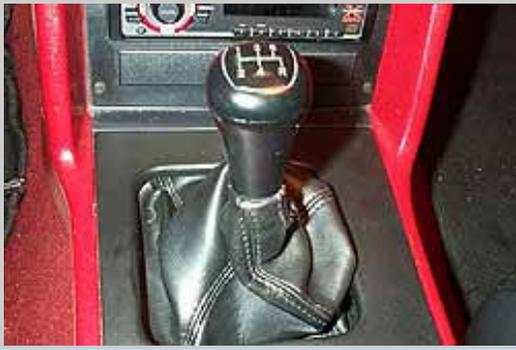
**13** The leather boot and trim cover are put back in place. It's a shame we have to hide the shiny billet steel, but its a major relief knowing we can shift without the fear of missing a gear or breaking a shift fork.
