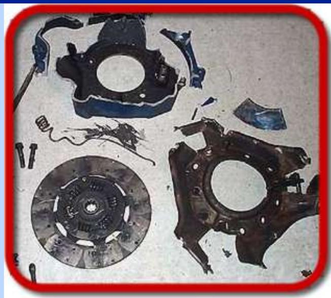
**Send in the bomb squad:** The entire aftermath of this clutch explosion can't even be seen in this photo. Shrapnel poked a hole in the hood, pinched a header collector in half, ripped the accelerator pedal right off the firewall, destroyed the shock tower brace, severed the main engine harness, and knocked out a freeze plug in the back of the block. It's amazing the driver wasn't injured.
