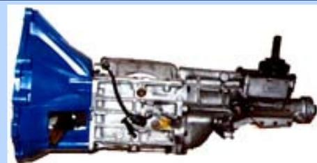
Seek out a T5 from a V8 car, ideally a Mustang. The 1983-1989 V8 T5's are rated at 265 lb.ft. of torque, while the 90-93 T5's are rated good to 300lb.ft. Typically these can be had for \$200-600 used. A new T5 will run about \$1000.
