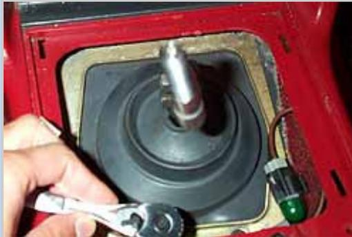
**2** Getting the dust boot off is one of the frustrating parts of the otherwise simple installation. The two screws at the back can be reached with a 1/4" drive ratchet and 11/32" socket on an extension. However the two front screws are hidden under the console, and will require patient removal, half-turn at a time, with a open end wrench.
