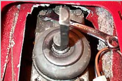
**3** With the dust boot removed and the swearing out of the way, we're ready to remove the shifter itself. Once again a sockets make easy work of the rear two bolts, but the front two require a wrench.
