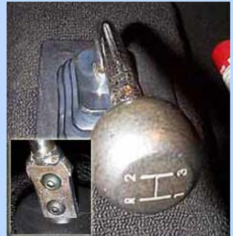
You can maintain the stock look by modifying the early shifter. We hacked off the 3spd/4spd lower bracket and welded on a metal tab. Drill two 3/8" holes to match the T5 shifter nub. Slip the stock boot over it and no one can tell from the inside that you've got an extra gear!
