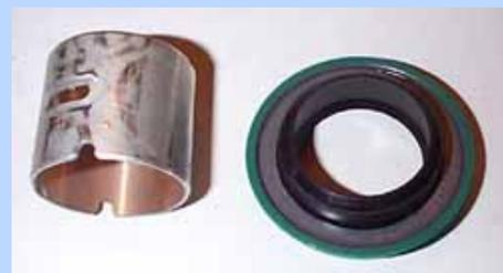
The tailshaft bushing and seal should be replaced if you bought your T5 transmission used, or if you are installing a new slip yoke. For more info on how to do this, [check here](#).
