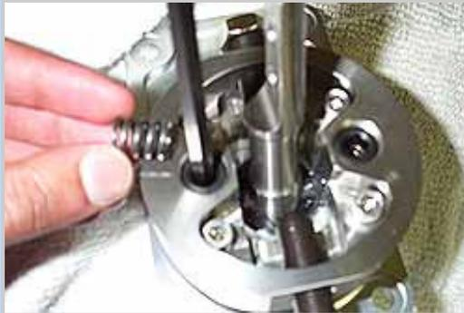
**8** Another feature of the Pro Ripper is the ability to change the stiffness of the neutral position. If you prefer more side-to-side resistance remove the allen plugs and swap out to the stiffer springs (included.) We left ours alone.
