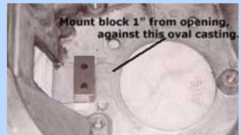
For early Fords with manual clutches, you'll need to install or transfer the fulcrum style clutch fork from a four speed or toplayer bellhousing. Due to the longer input shaft of the T5 you need the 1" spacer block under the fulcrum. Available from Windsor Fox, Mustangs Unlimited, and others.
