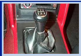
**13** The leather boot and trim cover are put back in place. It's a shame we have to hide the shiny billet steel, but its a major relief knowing we can shift without the fear of missing a gear or breaking a shift fork.
