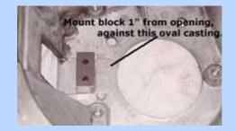
For early Fords with manual clutches, you'll need to install or transfer the fulcrum style clutch fork from a four speed or toploader bellhousing. Due to the longer input shaft of the T5 you need the 1" spacer block under the fulcrum. Available from Windsor Fox, Mustangs Unlimited, and others. The hair clip shown at the top holds the fork on the fulcrum, don't leave it out!
