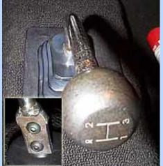
You can maintain the stock look by modifying the early shifter. We hacked off the 3spd/4spd lower bracked and welded on a metal tab. Drill two 3/8" holes to match the T5 shifter nub. Slip the stock boot over it and no one can tell from the inside that you've got an extra gear!
