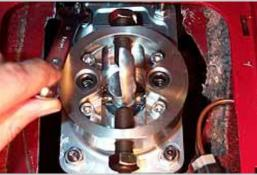
${\bf 10}$  With the new shifter positioned over the studs, the nuts and washers are secured evenly.
