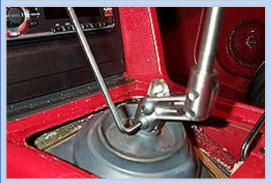
**11** The Pro Rippers two-piece stick offers a variety of mounting positions to suit your driving posture and vehicle configuration. We simply bolted the stick to the lower two mounting holes on the shifter to obtain about a 30% shorter throw than stock.
