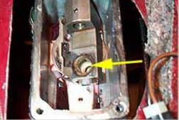
${\bf 6}$  Clean up the old silicone, and make sure none of it falls into the T5 (it'll clog up the fluid passages.)
