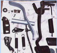
Converting an early Ford from automatic to manual requires rounding up the original clutch activation parts. This can be tough, the best bet is to find a wrecked four-speed car and take everything. Shown here are parts fro an early Mustang, including the z-bar
