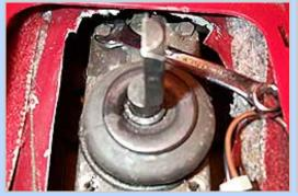
again a sockets make easy work of the rear two bolts, carved up transmission tunnel.) but the front two require a wrench.
