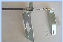
The kit is designed for strength as well as ease of installation. The 1/8" thick steel support plate mounts between the firewall and master cylinder. It not only locates the cable but strengthens the firewall by distributing the brake and clutch pedal loads.
