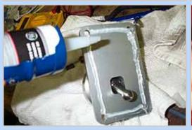
**9** Apply a thin bead of silicone between the bolt holes as shown. By the way, regular indoor-outdoor clear silicone works fine for everything on a car or engine, and costs a fraction of the RTV stuff.
