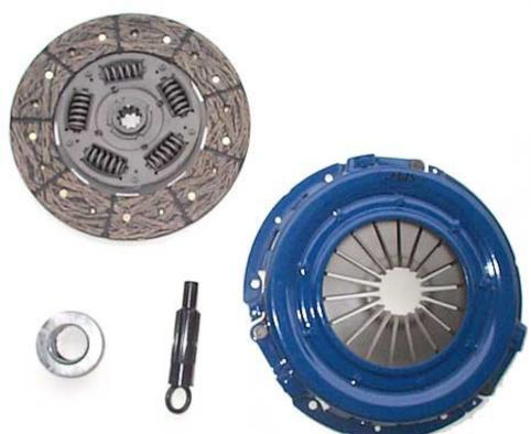
Selecting the proper clutch is a key ingredient of the T5 swap. You don't want to skimp here, otherwise you'll be doing the work all over again We talked to the clutch experts at <u>SPEC (Star Performance Engineered Clutches</u>), and they recommended their Stage 1 clutch, PN:SF481. Their stage 1 clutch will hold 300 horsepower with no problems, yet allow for chatterless engagement and low rpm driveability. At about \$159, including throwout bearing and alignment tool, the price is right too.
