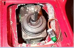
**3** With the dust boot removed and the swearing out of the way, we're ready to remove the shifter itself. Once we <u>converted to T5</u>(hence the green shifter light and
