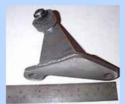
If you have a late 80's 5.0L block, you will need this piece from Windsor-Fox. It bolts to the bellhousing and provides a place for the stock "z bar" to mount. Early blocks had a threaded boss in the back of the block.
