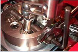
**12** The final step is to set the shifter stops. The shift forks in a T5 and T45 are weak and can bend if the shifter is slammed hard into gear. The stops prevent such over extension. Simply put the shifter in gear then turn in the large stop screw until it just makes contact with the shifter. Back it off 1/2 turn and lock it into place. Repeat for the other stop.
