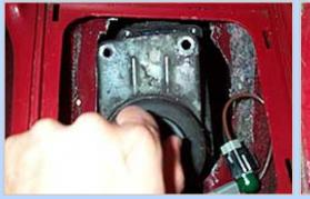
**5** With the four bolts removed, a little prying is all it takes to break the silicone bead holding the stock shifter to the T5.
